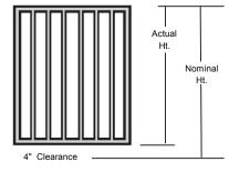
Frame:1-1/2" Square Frame, 14 Ga. - 3' to 9' Width<br/>2" Square Frame, 14 Ga. - 10' to 24 ' Width<br/>Hardware not includedPickets:3/4" or 1" Vertical Pickets, 16 Gauge<br/>Pickets Welded on Four Sides<br/>4-5/8 " Picket CentersFinish:Black Powder Coat - Standard<br/>Optional Colors Available
